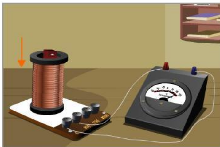
The North pole of the magnet is moved into the coil of wire
