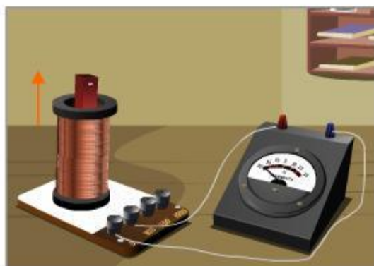
The North Pole of the Magnet is Moved out of the Coil of Wire
