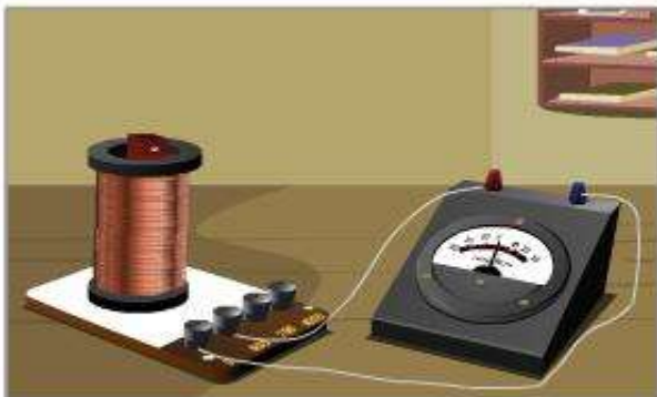
The Magnet is Held Stationary Inside the Coil of Wire
