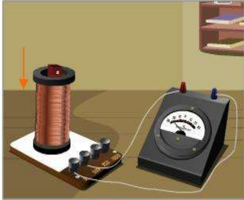
The South Pole of the Magnet is Moved into the Coil of Wire
